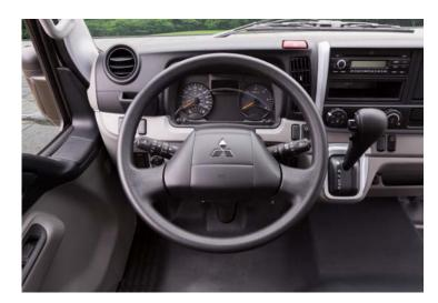
An infinitely adjustable steering wheel and dash-mounted shifter give drivers more control, while instruments and displays are always within easy reach or view. By moving the shifter off the floor, we create more leg room and easier access for passengers.
